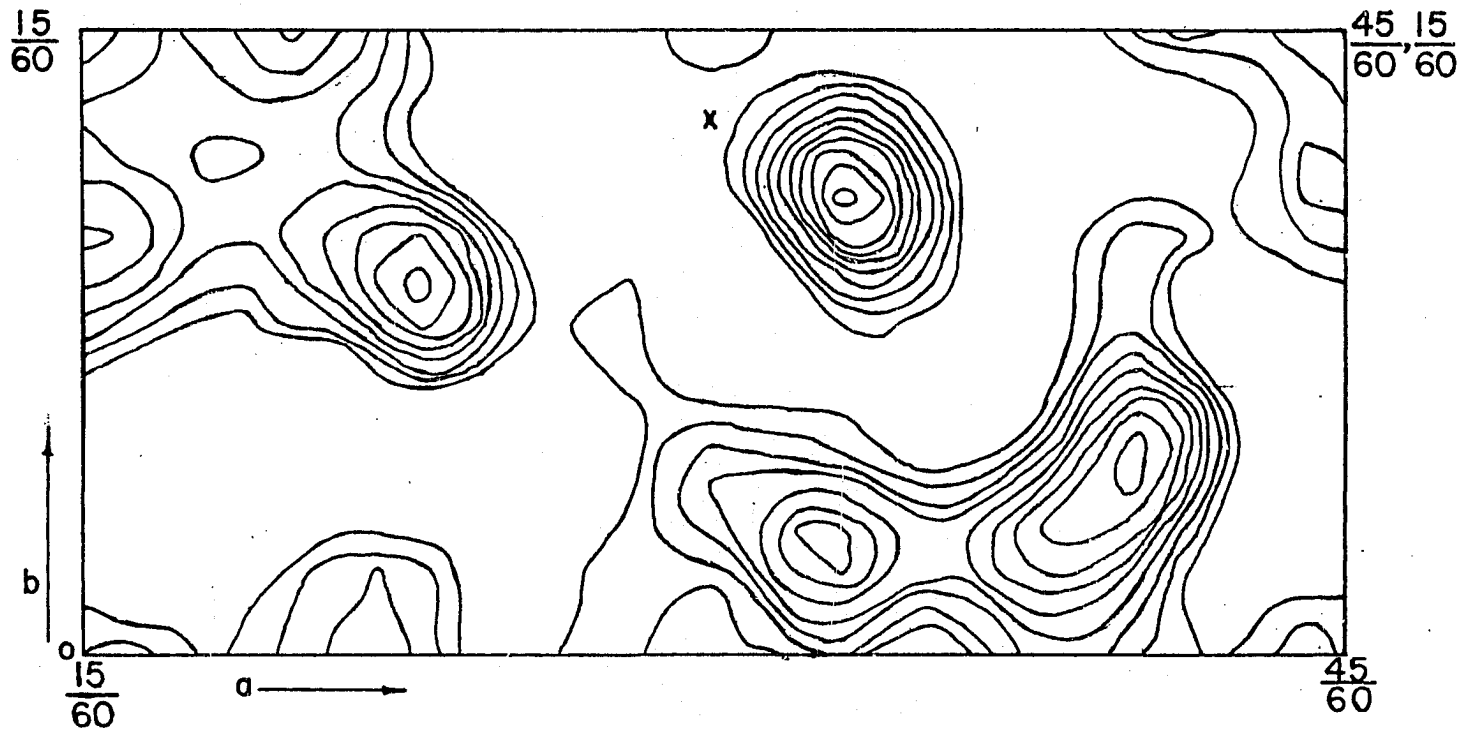
Figure 9. Partial difference electron density projection onto the (001) plane (only the metal atom contribution to the scattering has been subtracted out)
